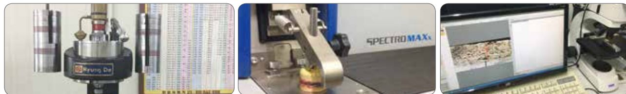
3 Checking composition and hardness during alloying
