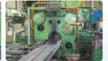
2,750Ton Extruding machine
