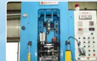
Graphite plugs press machine
