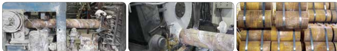
4 Billet by continuous casting and cutting
